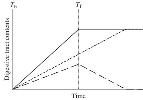
Fig. 1. Theoretical trajectories of stomach (---), gut (.....) and total digestive tract (—) of original Moriarty and Moriarty (1973) model assuming linear stomach evacuation and constant ingestion rate.  $T_b$  and  $T_f$  = begin and end of feeding phase, respectively
